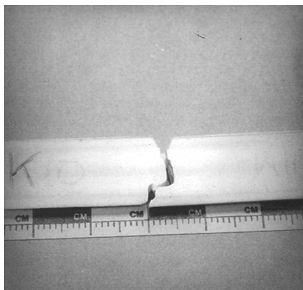
Figure 9 Brittle failure impact test bar.
